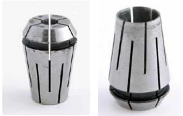
Scoring on collets that spun in the pocket due to inadequate holding power from the nut.
