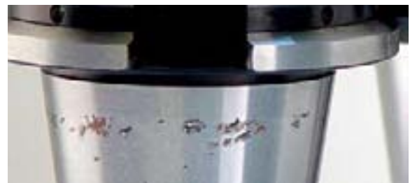
Fretting (wear marks) on a toolholder taper.
