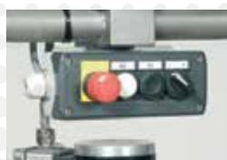
The sander is constructed as a two-hand machine where the controls are conveniently placed in between the handles. This makes it easy to regulate sanding direction, start/stop and emergency stop.
