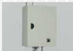
All electronics required by the Stack sander are contained in a wall-mounted box. For easy regulation of the sanding speed, the control button is placed on the outside of the box.
