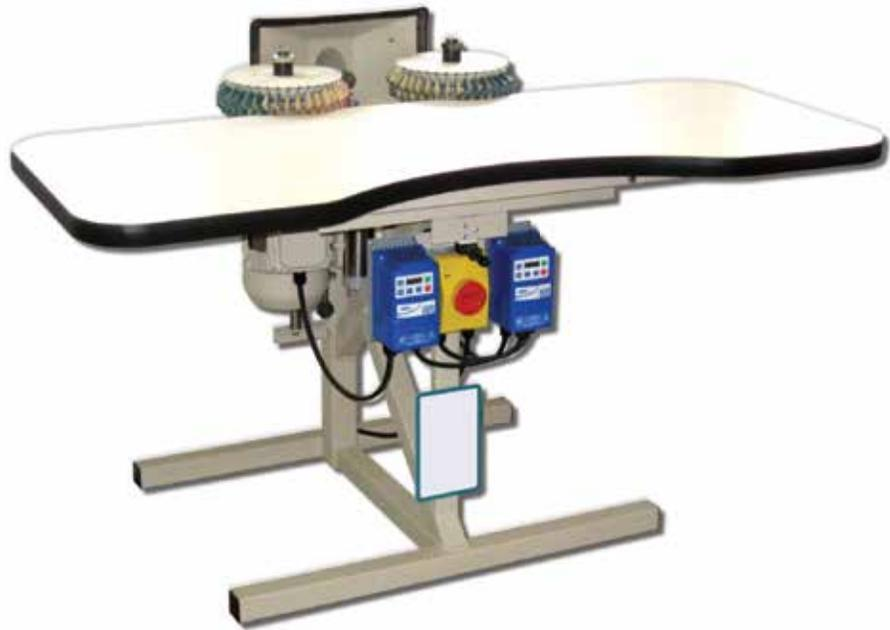
**THE 220 SERIES** features two counter-rotating spindles to be used with brush type sanding wheels. This allows parts to be sanded without noticeable rounding over on corners. The sanding technique is to sand the left corners on the right sander and the right corners on the left sander. This method has the brushes formed to the profile as they exit over the corners.
