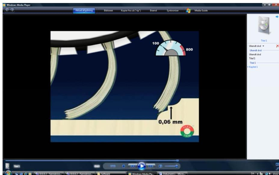
Low speed = better sanding in profiles – better edge-break – long lifetime on abrasives.
