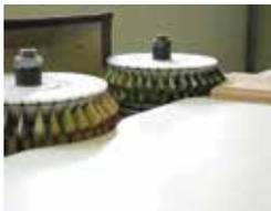
**SPINDLES LOWERED, TABLE FORWARD FOR EDGE SANDING**
